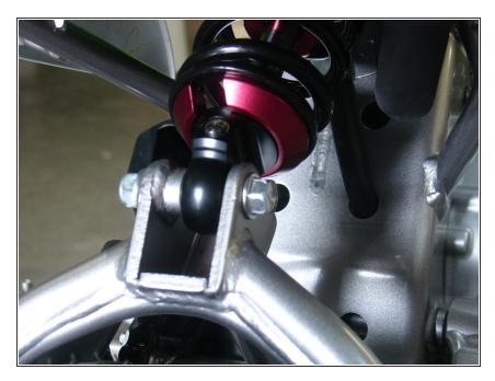
On Stage 2 models the rebound adjuster located on lower eyelet of the shocks should be oriented towards the rear of the vehicle, as shown. If needed, you can turn the lower eyelet to orient properly.
