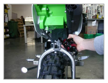
Install the new Elka shock with the head mounted at the top.
