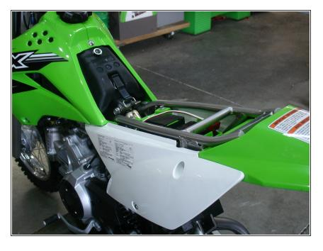
Remove the seat for better access to the top mounting bolt.
