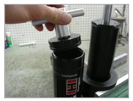
Screw the Elka tool (ASS-TL-0001) on the schrader valve threads and pull the rezzy cap out.
