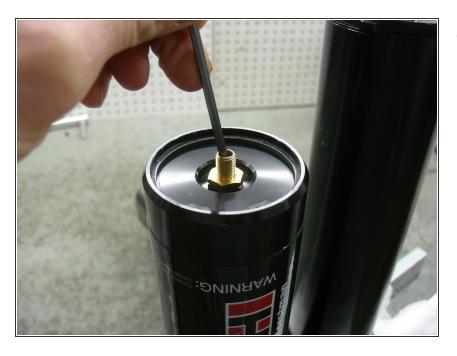
Release reservoir pressure by pushing the center core of the schrader valve. Be sure all the pressure is removed before performing the next step.
