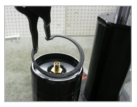
Using a proper circlip tool, remove the rezzy cap clip.
