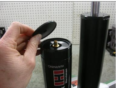
Unscrew and remove the rezzy cap protector with the Elka tool: LK-TL583.
