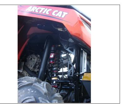
Install the front new Elka shocks with the reservoir (on Stage 3-4-5) or Schraeder nitrogen valve (on Stage 1-2) at the top of vehicle. ( right side shown).
