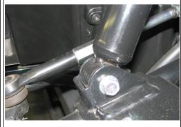
• Remove the top and bottom shock bolts and then remove the stock shock.
