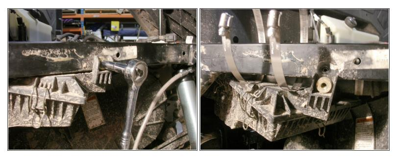
Remove the bolt holding the air box to allow enough clearance to slide in the provided reservoir collars.
