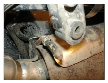
• Detach the muffler from its 2 rubber attachments to facilitate the routing of the hose.
