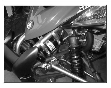
The front reservoirs must be secured to the front of the frame, right underneath the fender. The compression knobs must face towards outside of the quad.
