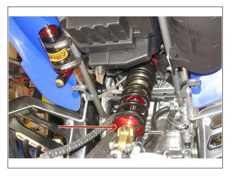
The rebound adjuster (adjustable using a screwdriver) located at the bottom of the shock should face the
