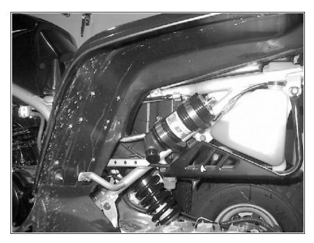
The rear reservoir must be attached to the rear sub-frame on the left side of the quad, right underneath the fender.
