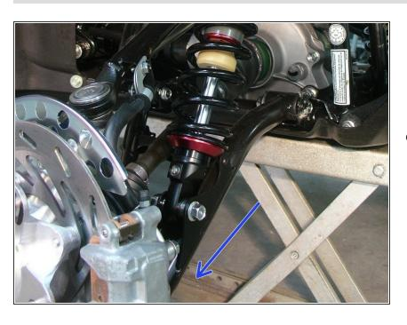
On Stage 2, Stage 4 and Stage 5 models, the lower shock eyelets should be installed with the rebound adjuster oriented towards the outside of the vehicle as shown by the blue Arrow on the photo ( right side shown ). If needed, you can turn the lower eyelet to orient properly.
