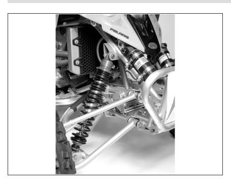
The front reservoirs must be secured to the front of the frame, right underneath the fender.
