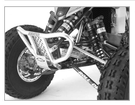
The rear reservoir must be attached to the front of the frame on the left side of the quad, right underneath the fender. The compression knobs must face towards the side of the quad.
