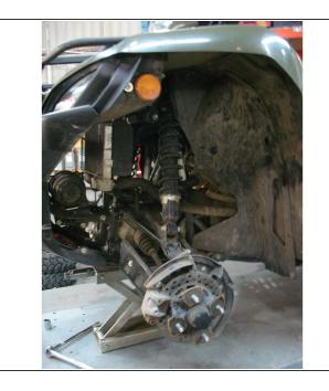
Lift the vehicle using a jack or stand so that the wheels are off the ground. Refer to your vehicle's owner manual for specific instructions on how to remove the stock shocks. Keep your original bolts to re-use when installing your new Elka shocks.
