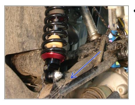
On Stage 2, Stage 4 and Stage 5 models, the lower shock eyelets should be installed with the rebound adjuster oriented towards the outside of the vehicle as shown by the blue Arrow on the photo ( right side shown ). If needed, you can turn the lower eyelet to orient properly.
