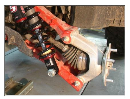
On Stage 2, Stage 4, and Stage 5 models the rebound adjuster located on lower eyelet of the shocks should be oriented towards the rear of the vehicle, as shown. (right side shown ). If needed, you can turn the lower eyelet to orient properly.
