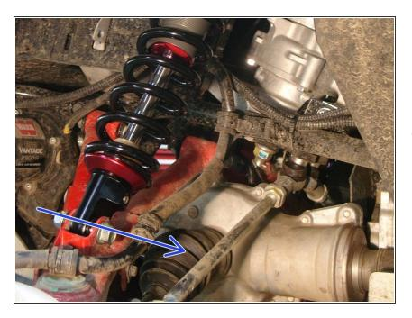
On Stage 2, Stage 4 and Stage 5 models, the lower shock eyelets should be installed with the rebound adjuster oriented towards the rear of the vehicle as shown by the blue Arrow on the photo ( left side shown ). If needed, you can turn the lower eyelet to orient properly.
