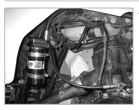
The rear reservoir must be attached to the front of the frame on the left side of the quad, right underneath the fender. The compression knobs must face the front of the quad.
