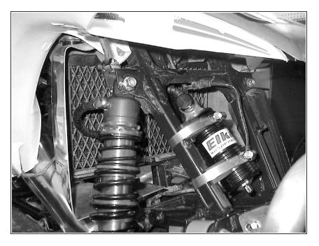
The front & rear reservoirs must be secured to the front of the frame, right underneath the fender.
