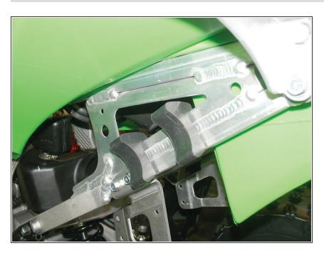
Install the provided rubber mounts on the left side of the rear subframe with the tab on top.
