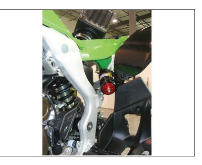
Route the reservoir's hose above the small airbox chamber, pulling out the reservoir through the left side of the rear subframe. Attach the shock to the upper mount using the stock bolts.
