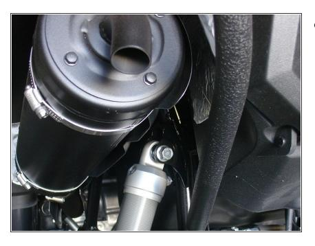
On Stage 1 and Stage 2, the left and the right shock are the same. Install them with the shraeder nitrogen valve at the top of vehicle, with the valve towards the Inside of the vehicle ( left side shown ).
