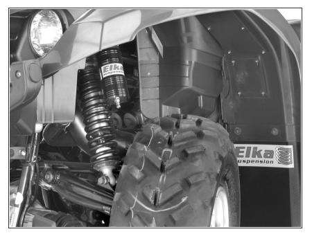
• The piggyback reservoirs should be at the top of the shocks when installed, with the adjustment knob facing towards the outside of the quad.
