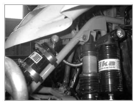
The rear reservoir must be attached to the front of the frame on the left side of the quad, right underneath the fender. The compression knobs must face towards outside of the quad.
