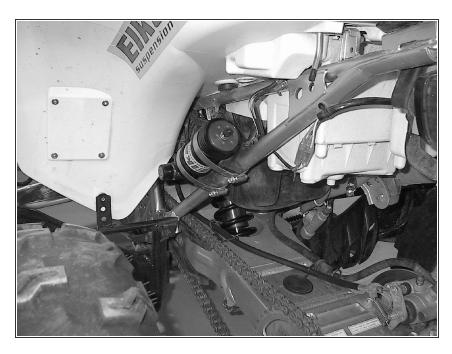
The rear reservoir must be attached to the rear subframe on the left side of the quad, right underneath the fender. The compression knobs must face towards the side of the quad.
