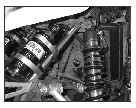
The front reservoirs must be secured to the front of the frame, right underneath the fender.
