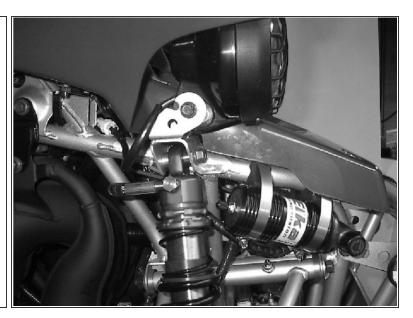
The banjo bolts must be oriented towards the sides of the vehicle with the hose coming out towards the rear. The reservoirs must be attached to the front of the frame using the provided rubber holders and metal collars. Make sure to route the hoses according to photos.
