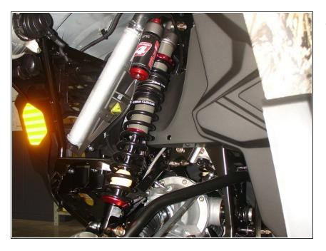
Install the front new Elka shocks with the reservoir (on Stage 3-4-5) or Schraeder nitrogen valve (on Stage 1-2) at the top of vehicle. ( left side shown).
