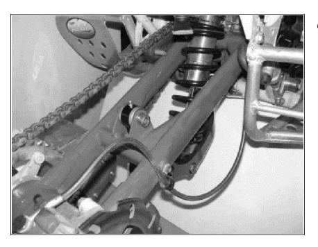
Install the black part of the Dual-Linkage and attach it to the swingarm.
