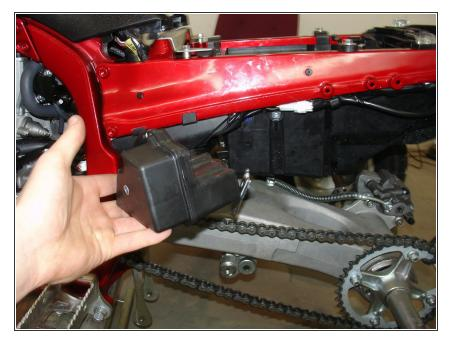
• Remove the overflow oil tank.
