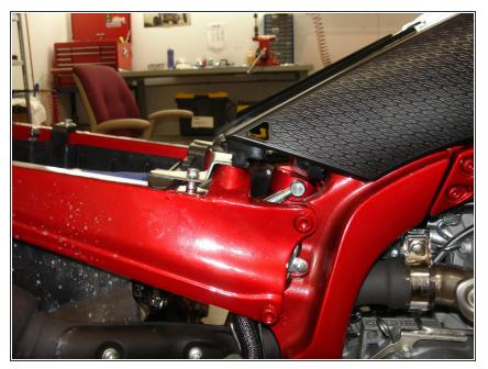
• The hose needs to be on the right side of the quad when you install the upper bolt on the suspension.
