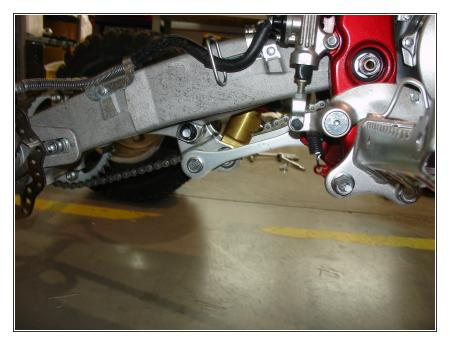
Install the linkage and put the rebound adjuster (adjustable using a screwdriver) at the bottom of the shock should face the front of the quad.
