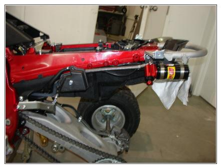
• Pass the rear hose near the sub frame and install overflow oil tank.
