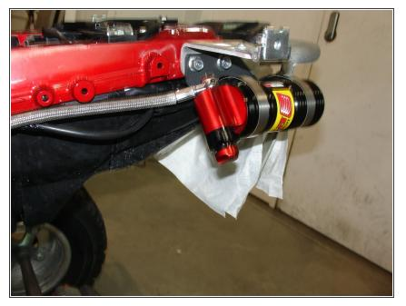
Install the rubber mount on the rear bracket and the reservoir with the angle as shown (install the rear fenders before tighten the rear reservoir).
