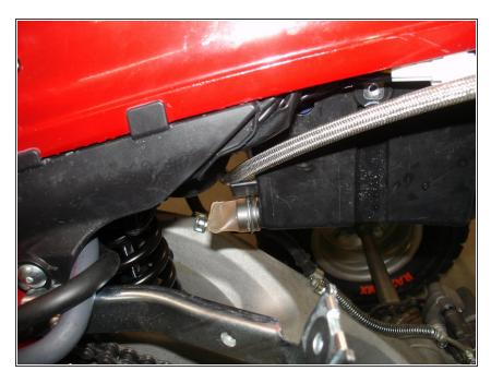
• Pass the hose between the intake system and the air box.
