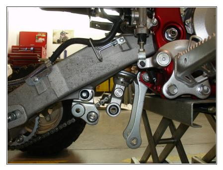
• Remove the linkage bolt and the upper shock bolt.
