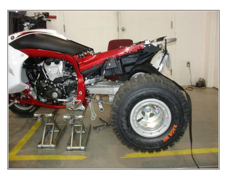
Remove the stock suspension. You need to lift the axle. You can use a strap.
