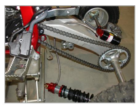
• To install the ELKA shock, you need to pass the reservoir in the swing arm first.
