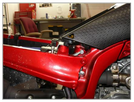
• The hose needs to be on the right side of the quad when you install the upper bolt on the suspension.
