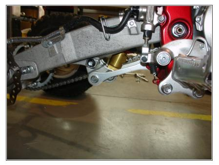
Install the linkage and put the rebound adjuster (adjustable using a screwdriver) at the bottom of the shock should face the front of the quad.
