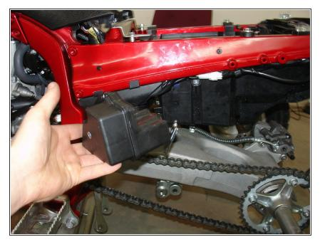
• Remove the overflow oil tank.
