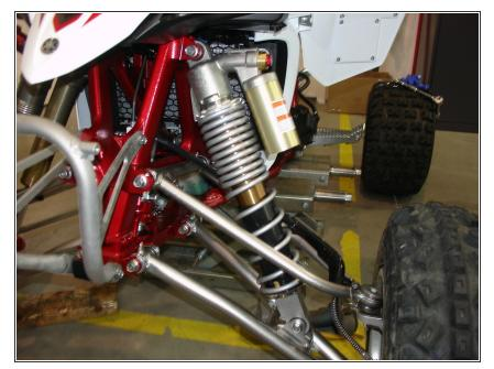
Lift the vehicle off the ground with a jack or on a stand. Remove the stock shock absorbers from the vehicle.
