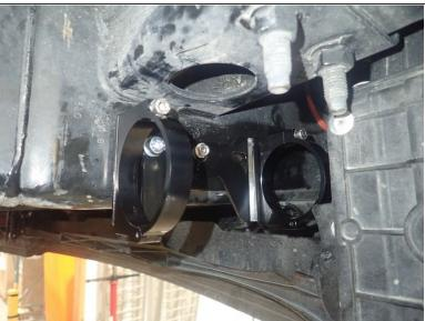
Orienting the bracket assembly as horizontally as possible, use the supplied self-taping screw to secure the bracket in the center bracket hole.
