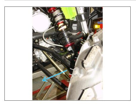
On Stage 2, Stage 4 and Stage 5 models, the lower shock eyelets should be installed with the rebound adjuster oriented towards the rear of the vehicle as shown by the blue arrow on the photo (right side shown). If needed, you can turn the lower eyelet to orient properly. This will facilitate access to the adjuster.
