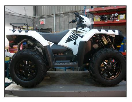
Lift the vehicle using a jack or stand so that the wheels are off the ground. Refer to your vehicle's owner manual for specific instructions on how to remove the stock shocks. Keep you original bolts to re-use when installing your new Elka shocks.
