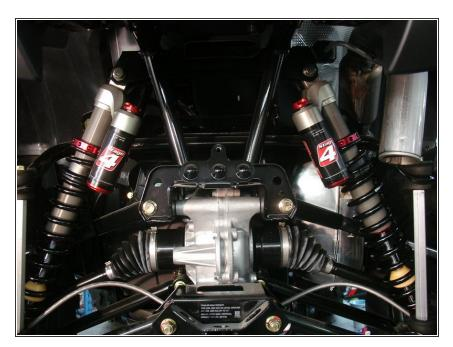
Install the new Elka rear shocks with the piggyback reservoir at the top and oriented towards the rear of the vehicle and pointed slightly inside the vehicle.
