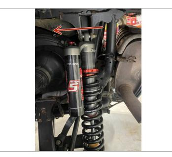
Install the left and right new Elka rear shock with the piggyback reservoir at the top and oriented towards the front of the vehicle as indicated by the red Arrow on the photo.
