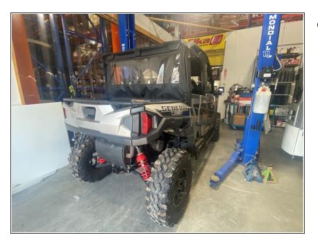
Lift the vehicule using a jack or stand so that the wheels are off the ground. Refer to your vehicule's owner's manual for specific instructions on how to remove the stock shocks. Keep the Original bolts to re-use when installing your nes Elka Shocks
