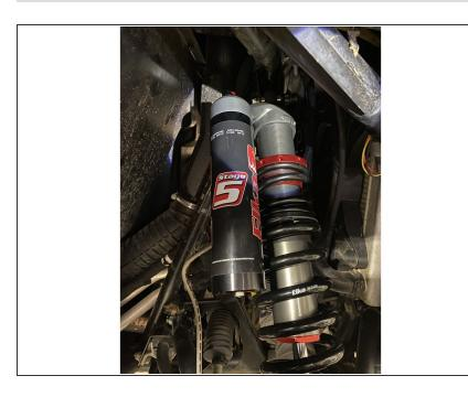
Install the front new Elka shocks with the reservoir (on Stage 3-4-5)
