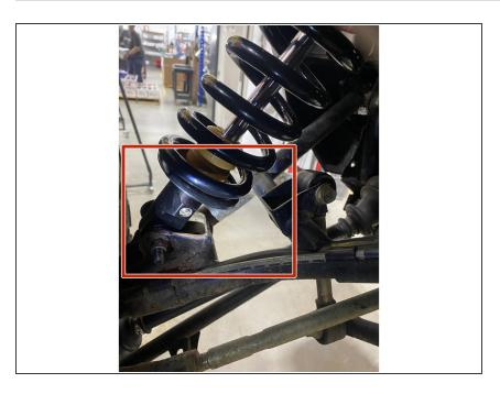
On Stage 2, Stage 4 and Stage 5 models, the lower shock eyelets should be installed with the rebound adjuster (red square) oriented towards the back of the vehicle as shown by the Red square on the photo (left side shown). If needed, you can turn the lower eyelet to orient properly.
