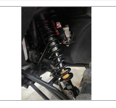
Insert wisdom here.Install the front new Elka shocks with the reservoir ( on Stage 3-4-5 ) left side shown .
