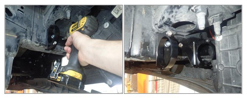
Orienting the bracket assembly as horizontally as possible, use the supplied self-taping screw to secure the bracket in the center bracket hole.
