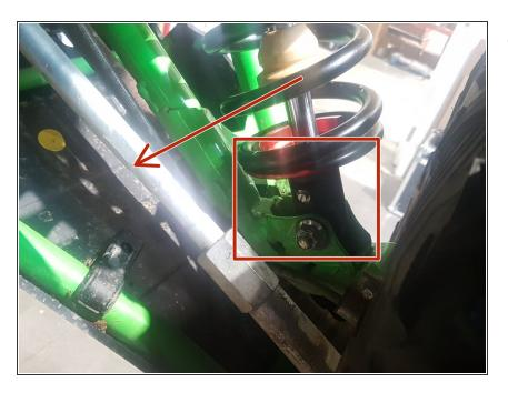
The lower shock eyelets should be installed with the rebound adjuster (red square) oriented towards the back of the vehicle as shown by the Red square on the photo ( Right side shown). If needed, you can turn the lower eyelet to orient properly.
