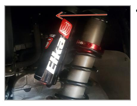
Install the left and right new Elka rear shock with the piggyback reservoir at the top and oriented towards the rear of the vehicle as indicated by the red Arrow on the photo.
