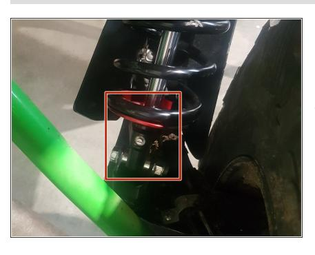
The rebound adjuster located on lower eyelet of the shocks should be oriented towards the rear of the vehicle, as shown. (Shown by the red square). If needed, you can turn the lower eyelet to orient properly.
