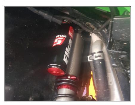
Install the front new Elka shocks ( Right side shown). The reservoir must be orientated outwards
