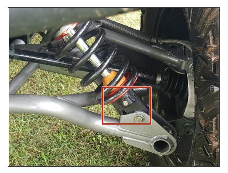
On Stage 2, Stage 4, and Stage 5 models the rebound adjuster located on lower eyelet of the shocks should be oriented towards the rear of the vehicle, as shown. (Shown by the red square ). If needed, you can turn the lower eyelet to orient properly.
