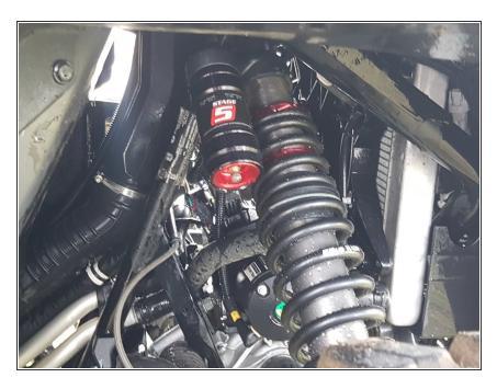
Install the front new Elka shocks with the reservoir ( on Stage 3-4-5 ) Right side shown . The reservoir must be orientated backwards
