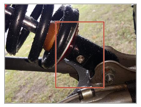
On Stage 2, Stage 4 and Stage 5 models, the lower shock eyelets should be installed with the rebound adjuster (red square) oriented towards the back of the vehicle as shown by the Red square on the photo (Right side shown). If needed, you can turn the lower eyelet to orient properly.
