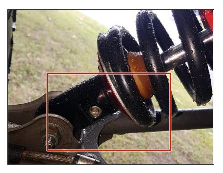
On Stage 2, Stage 4 and Stage 5 models, the lower shock eyelets should be installed with the rebound adjuster (red square) oriented towards the back of the vehicle as shown by the Red square on the photo (left side shown). If needed, you can turn the lower eyelet to orient properly.
