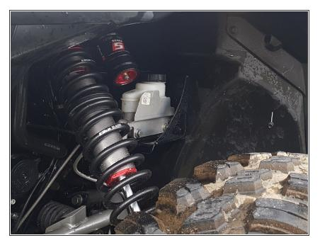
Insert wisdom here.Install the front new Elka shocks with the reservoir ( on Stage 3-4-5 ) left side shown . The reservoir must be orientated backwards
