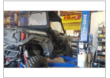
Lift the vehicule using a jack or stand so that the wheels are off the ground. Refer to your vehicule's owner's manual for specific instructions on how to remove the stock shocks. Keep the Original bolts to re-use when installing your nes Elka Shocks
