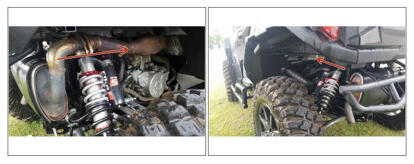
Install the left and right new Elka rear shock with the piggyback reservoir at the top and oriented towards the front of the vehicle as indicated by the red Arrow on the photo.
