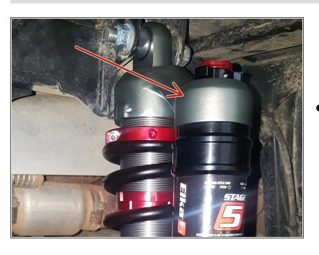
Install both new Elka rear shock with the piggyback reservoir at the top and oriented outwards to the side of the vehicule as indicated by the red Arrow on the photo. On Stage 1 and Stage 2, the left and the right shock are the same. Just install them with the shraeder nitrogen valve at the top of vehicle.
