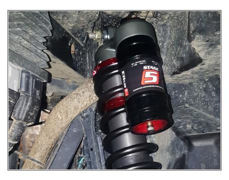
• Install the front new Elka shocks with the reservoir (on Stage 3-4-5) at the top of vehicle and facing outwards of vehicle (right side shown). Install the front new Elka shocks (on stage 1 and 2) with the Schraeder nitrogen valve at the top of vehicle.
