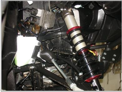
Install the front new Elka shocks with the reservoir (on Stage 3-4-5) at the top of vehicle and facing outwards of vehicle (right side shown). Install the front new Elka shocks (on stage 1 and 2) with the Schraeder nitrogen valve at the top of vehicle.
