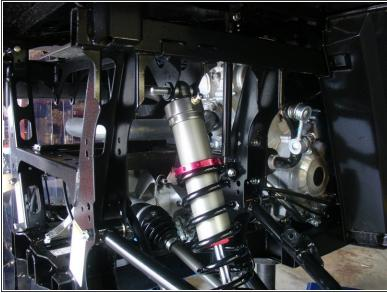
Install both new Elka rear shock with the piggyback reservoir at the top and oriented forward to
