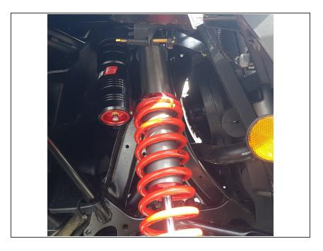
Install the front new Elka shocks with the reservoir (on Stage 3-4-5) or Schraeder nitrogen valve (on Stage 1-2) at the top of vehicle. ( Right side shown). The reservoir must be orientated backwards
