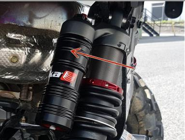
• Install the left and right new Elka rear shock with the piggyback reservoir at the top and oriented towards the front of the vehicle as indicated by the red Arrow on the photo. On Stage 1 and Stage 2, the left and the right shock are the same. Just install them with the shraeder nitrogen valve at the top of vehicle.
