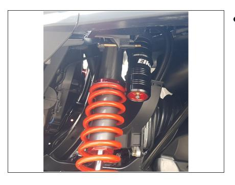
Insert wisdom here.Install the front new Elka shocks with the reservoir (on Stage 3-4-5) or Schraeder nitrogen valve (on Stage 1-2) at the top of vehicle. (left side shown ). The reservoir must be orientated backwards
