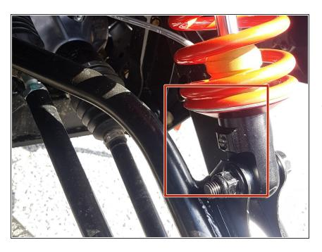
On Stage 2, Stage 4 and Stage 5 models, the lower shock eyelets should be installed with the rebound adjuster (red square) oriented towards the back of the vehicle as shown by the Red square on the photo (Right side shown). If needed, you can turn the lower eyelet to orient properly.
