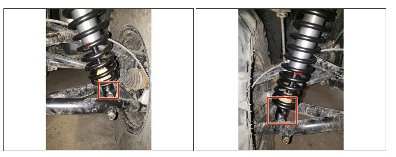
• On Stage 2, Stage 4, and Stage 5 models the rebound adjuster located on lower eyelet of the shocks should be oriented towards the rear of the vehicle, as shown. (Shown by the red square ). If needed, you can turn the lower eyelet to orient properly.
