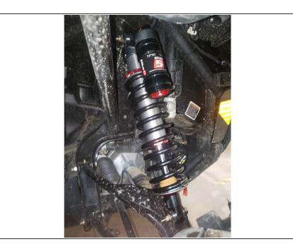
Install the front new Elka shocks with the reservoir (on Stage 3-4-5) or Schraeder nitrogen valve (on Stage 1-2) at the top of vehicle. ( Right side shown). The reservoir must be orientated outwards
