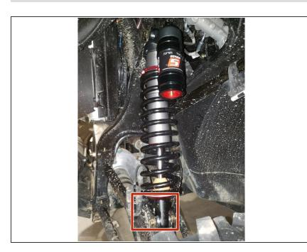
On Stage 2, Stage 4 and Stage 5 models, the lower shock eyelets should be installed with the rebound adjuster (red square) oriented towards the back of the vehicle as shown by the Red square on the photo (Right side shown). If needed, you can turn the lower eyelet to orient properly.
