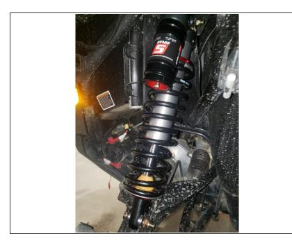
Install the front new Elka shocks with the reservoir (on Stage 3-4-5) or Schraeder nitrogen valve (on Stage 1-2) at the top of vehicle. ( left side shown). The reservoir must be orientated outwards.
