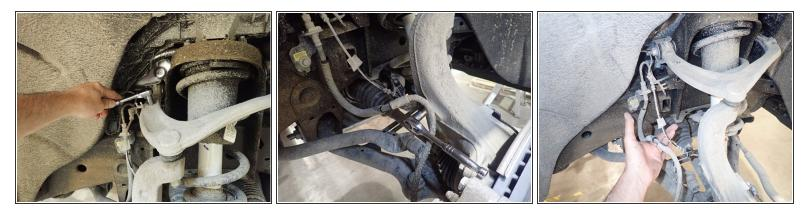
• Remove the bolts that hold the brake line on each side to make sure you don't damage them during installation.
