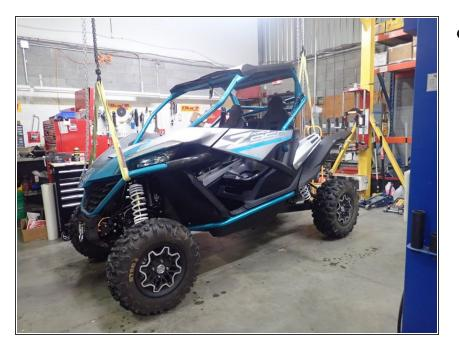
Lift the vehicle using a jack or stand so that the wheels are off the ground. Refer to your vehicle's owner manual for specific instructions on how to remove the stock shocks. Keep your original bolts to re-use when installing your new Elka shocks.
