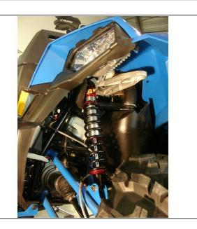
• Install the front new Elka shocks with the reservoir (on Stage 3-4-5) or Schraeder nitrogen valve (on Stage 1-2) at the top of vehicle. (left side shown).
