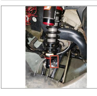
On Stage 2, Stage 4 and Stage 5 models, the lower shock eyelets should be installed with the rebound adjuster oriented towards the back of the vehicle as shown by the Red square on the photo ( Right side shown). If needed, you can turn the lower eyelet to orient properly.
