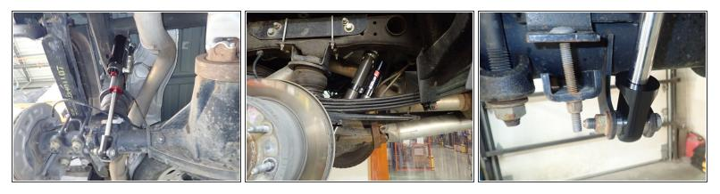
• Remove upper and lower bolts from OEM shocks. Keep OEM bolts to install Elka shocks.
