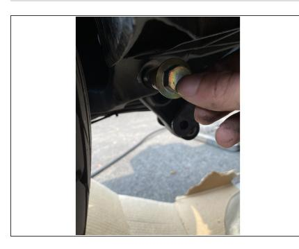
Use an impact or long breaker bar to remove the top linkage bolt (gold). This bolt is very tight
