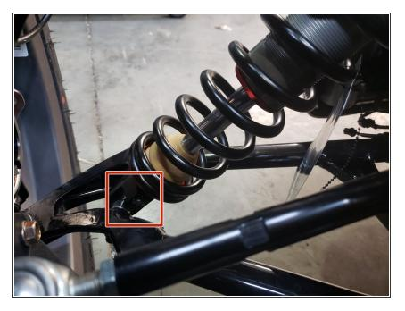
On Stage 2, Stage 4 and Stage 5 models, the lower shock eyelets should be installed with the rebound adjuster oriented towards the back of the vehicle as shown by the Red square on the photo ( Left side shown). If needed, you can turn the lower eyelet to orient properly.
