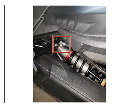
• Torque the top shock bolt to 20-26 ft.lbs
