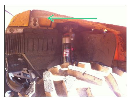
Install the <u>right</u> new Elka rear shock with the piggyback reservoir at the top and oriented towards
