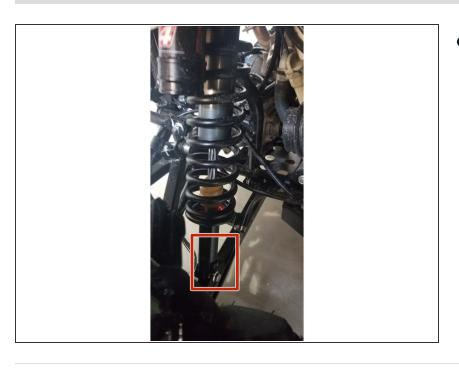
On Stage 2, Stage 4, and Stage 5 models the rebound adjuster located on lower eyelet of the shocks should be oriented towards the front of the vehicle, as shown. (Right side shown). If needed, you can turn the lower eyelet to orient properly.
