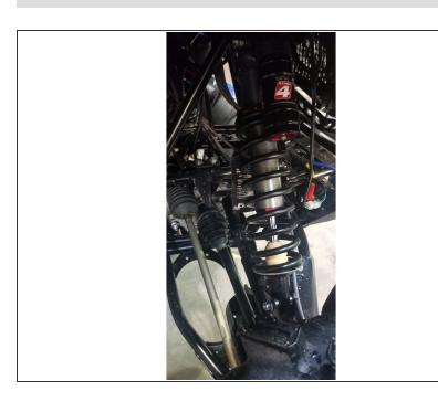
Install the front new Elka shocks with the reservoir (on Stage 3-4-5) or Schraeder nitrogen valve (on Stage 1-2) at the top of vehicle. ( Right side shown).
