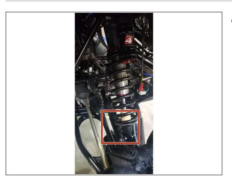
On Stage 2, Stage 4 and Stage 5 models, the lower shock eyelets should be installed with the rebound adjuster oriented towards the back of the vehicle as shown by the red square on the photo (Right side shown). If needed, you can turn the lower eyelet to orient properly.
