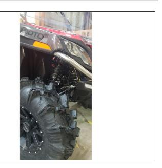
Lift the vehicle using a jack or stand so that the wheels are off the ground. Refer to your vehicle's owner manual for specific instructions on how to remove the stock shocks. Keep your original bolts to re-use when installing your new Elka shocks.
