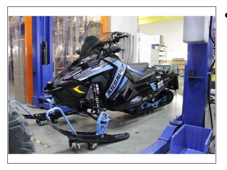
Lift the vehicle using a jack or stand so that the skis and track are off the ground. Refer to your vehicle's owner manual for specific instructions on how to remove the stock shocks. Keep your original bolts to re-use when installing your new Elka shocks.
