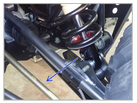
On Stage 2, Stage 4 and Stage 5 models, the lower shock eyelets should be installed with the rebound adjuster oriented towards the rear of the vehicle as shown by the blue Arrow on the photo ( Right side shown). If needed, you can turn the lower eyelet to orient properly.
