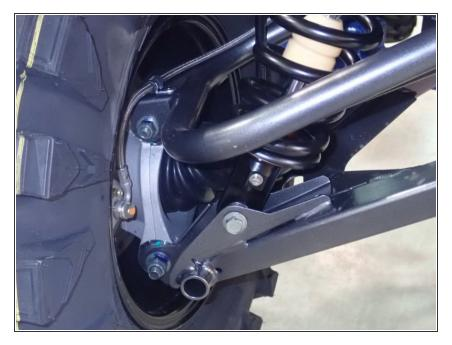
On Stage 2, Stage 4, and Stage 5 models the rebound adjuster located on lower eyelet of the shocks should be oriented towards the rear of the vehicle, as shown. (Leftt side shown). If needed, you can turn the lower eyelet to orient properly.
