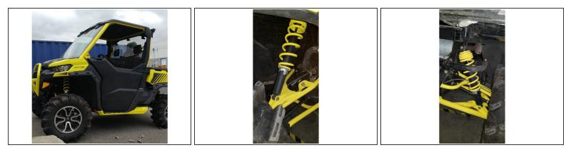
• Lift the vehicle using a jack or stand so that the wheels are off the ground. Refer to your vehicle's owner manual for specific instructions on how to remove the stock shocks. Keep your original bolts to re-use when installing your new Elka shocks.
