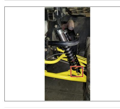
On Stage 2, Stage 4, and Stage 5 models the rebound adjuster located on lower eyelet of the shocks should be oriented towards the rear of the vehicle, as shown. (Right side shown ). If needed, you can turn the lower eyelet to orient properly.
