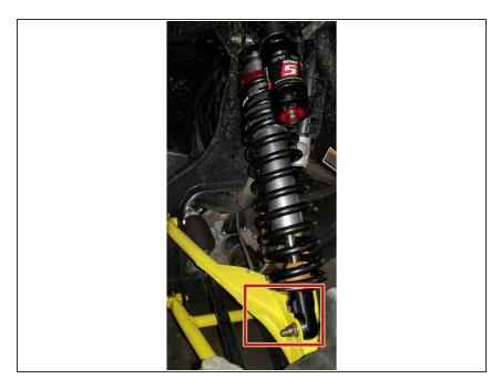
On Stage 2, Stage 4 and Stage 5 models, the lower shock eyelets should be installed with the rebound adjuster oriented towards the back of the vehicle as shown by the Red square on the photo ( Right side shown). If needed, you can turn the lower eyelet to orient properly.
