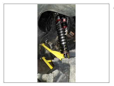
Install the front new Elka shocks with the reservoir ( on Stage 3-4-5 ) or Schraeder nitrogen valve ( on Stage 1-2 ) at the top of vehicle. ( Right side shown ).
