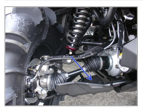
On Stage 2, Stage 4 and Stage 5 models, the lower shock eyelets should be installed with the rebound adjuster oriented towards the front of the vehicle as shown by the blue Arrow on the photo (Right side shown). If needed, you can turn the lower eyelet to orient properly.
