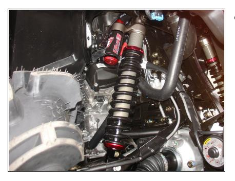
Install the front new Elka shocks with the reservoir (on Stage 3-4-5) or Schraeder nitrogen valve (on Stage 1-2) at the top of vehicle. ( Right side shown).
