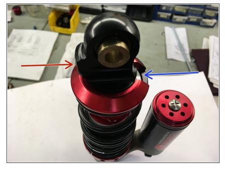
Before installing the front shock, rebound adjuster must be position at 180° (red arrow) of the reservoir and the spring slot (blue arrow) be in line with the reservoir as shown on the pictures.
