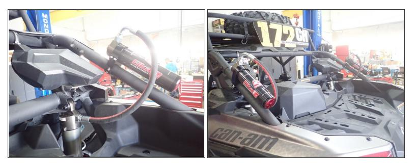
• The reservoir is attache to the cage at the top with the hose facing upward.
