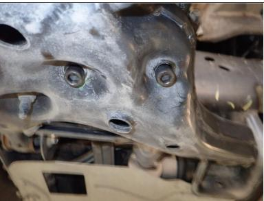
Install supplied upper bolts and washers, then do the same for lower mounting bolts. Tighten all bolts.
