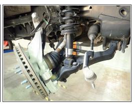
Remove upper arm ball joint nut and tie rod end ball joint nut, then separate them from steering knuckle.
