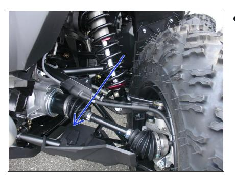
On Stage 2, Stage 4 and Stage 5 models, the lower shock eyelets should be installed with the rebound adjuster oriented towards the front of the vehicle as shown by the blue Arrow on the photo (left side shown). If needed, you can turn the lower eyelet to orient properly.
