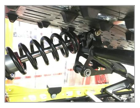
Installed the bottom shock mount in the elka linkage with the rebound adjuster facing upward.
