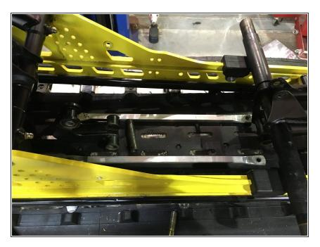
Remove the stock rear shock with both aluminium link.
