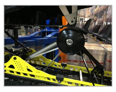
remove the two bolts that hold the rear skid.
