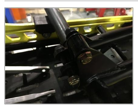
installed the elka linkage on the rear shock arm, use the stock shock bolt.
