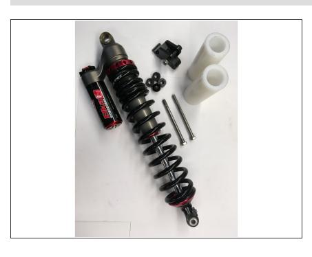
The Kit include:1 linkage, 2 long M8 bolts, 1 M8 shock bolt with lock nut, 4 aluminium spacers and 2 nylon sleeves
