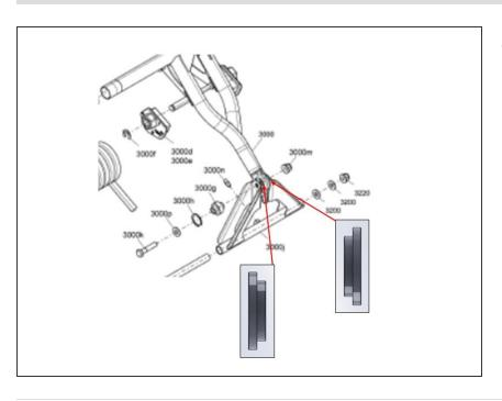
Install the provided t-motion delete bushing between rear arm assembly and the pivot arm.
