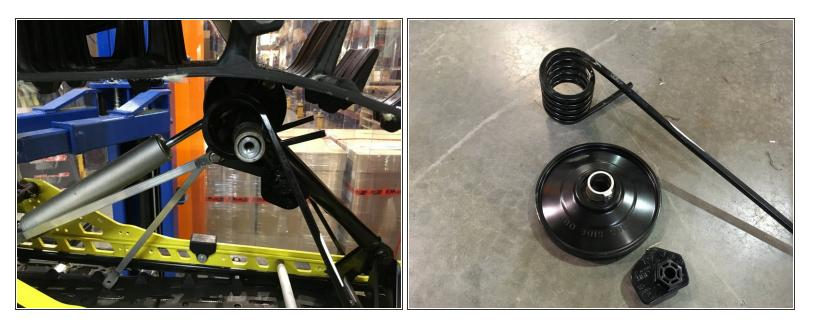
• Remove the Idler wheel, the torsion spring and the spring adjuster on both side.
